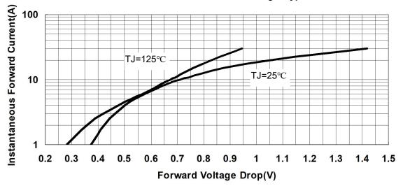
Fig.3-Typical Forward Voltage Drop Characteristics
